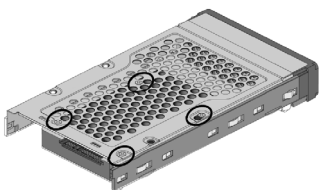
Figure 2-15-1. Installing 2.5-inch SAS/SATA Drive
