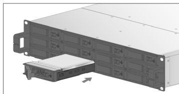
Figure 2-10. Installing Drive into Subsystem
