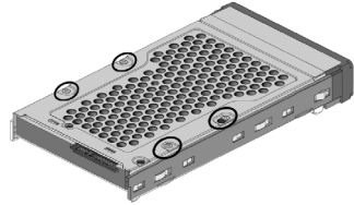
Figure 1-4-2. Installing 3.5-inch SAS/SATA Drive
